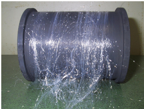
Fig. 7. Fibers derived from polymers prepared at 140–150 °C.
